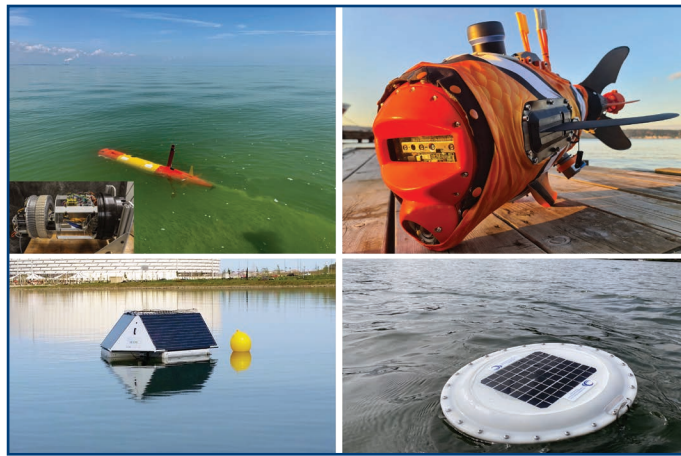
FIGURE 4. A variety of in situ sensors used to monitor HABs. Top left: A third-generation ESP (shown in bottom left of photo) from MBARI prior to its placement in a long-range autonomous underwater vehicle (LRAUV) and MBARI's LRAUV travelling across the surface of Lake Erie during a large algal bloom (photos: Ben Yair Raanan 2019, MBARI 2018). Top right: The MAZU, an untethered robot fish from the Aquaai Corporation (photo: Liane Thompson, www.aquaai.com/ ). Bottom left: The MPC Buoy from LG Sonic (photo: www.lgsonic.com/nysdec-will-use-mpc-buoys-to-combat-algae/ ). Bottom right: The Algae Tracker from AquaRealTime (photo: www.algaetracker.com/how-it-works ).
